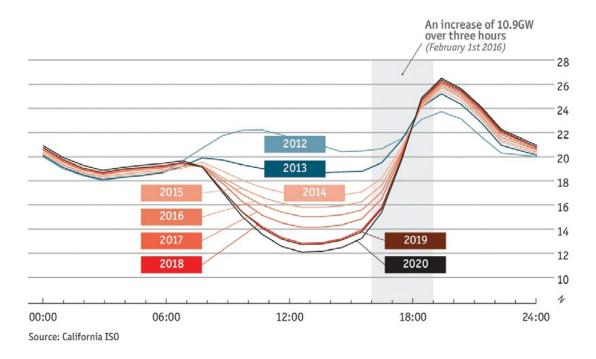
CAISO – Average electricity load requirement of a typical spring day in California<sup>17</sup>
