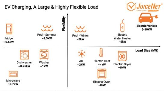
A typical 35-mile commute requires around 12.5 kWH of charging, which is 1-2 hours with our standard 10kW charging station.
